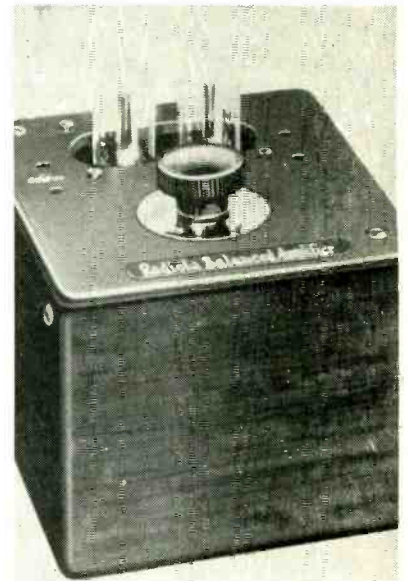
Development of this battery-operated two-tube amplifier in the early twenties made it possible to add a loudspeaker to the tuner so that the entire family could enjoy programs without headphones.
