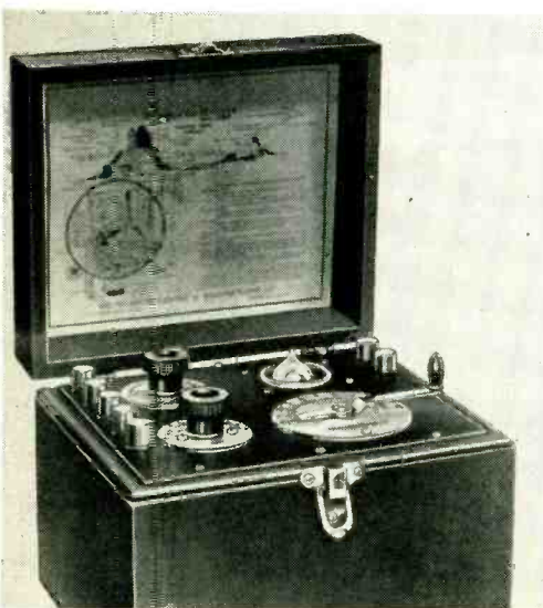
The Acriola Senior, Westinghouse's one-tube set using the WD-11 tube, went on the market in the early twenties. It ended the reign of the crystal receiver.
