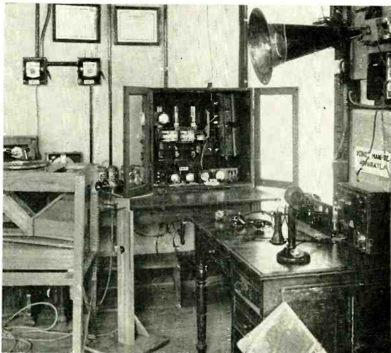
In 1921, J. W. Weed built this transmitter panel and operator's desk for KGW, Portland. At left is a home-made phonograph used for transmitting records; music had to be picked up by mike in front of phonograph.
