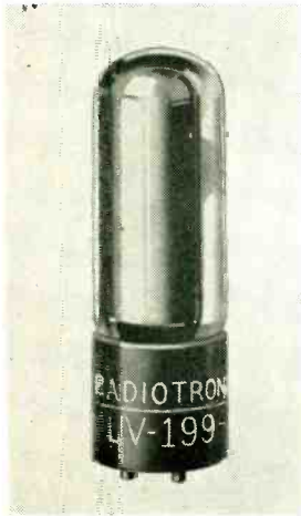
Portable radios became popular when RCA developed this battery-operated #99 tube.
