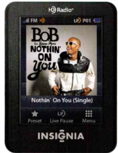
An Insignia portable HD Radio receiver, showing Artist Experience during a live broadcast.
