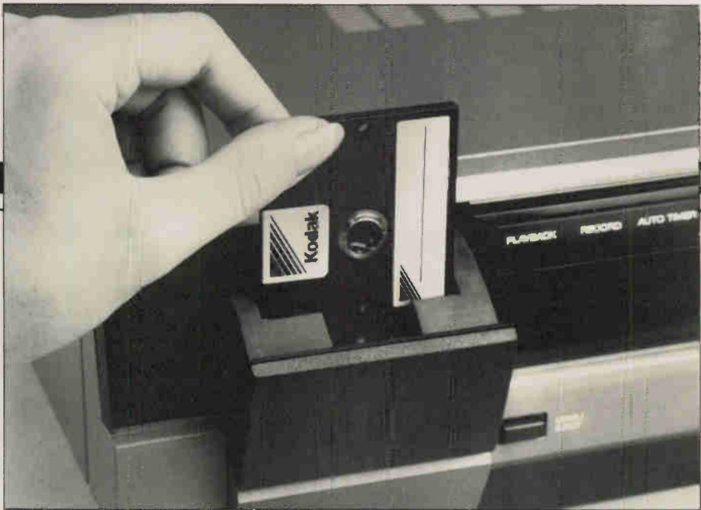
This is a close-up of Kodak's new video storage system that will allow you to display photographic images on TV sets. This video floppy-disk holds up to 50 images and... it's a lot smaller to file than a slide-tray!
