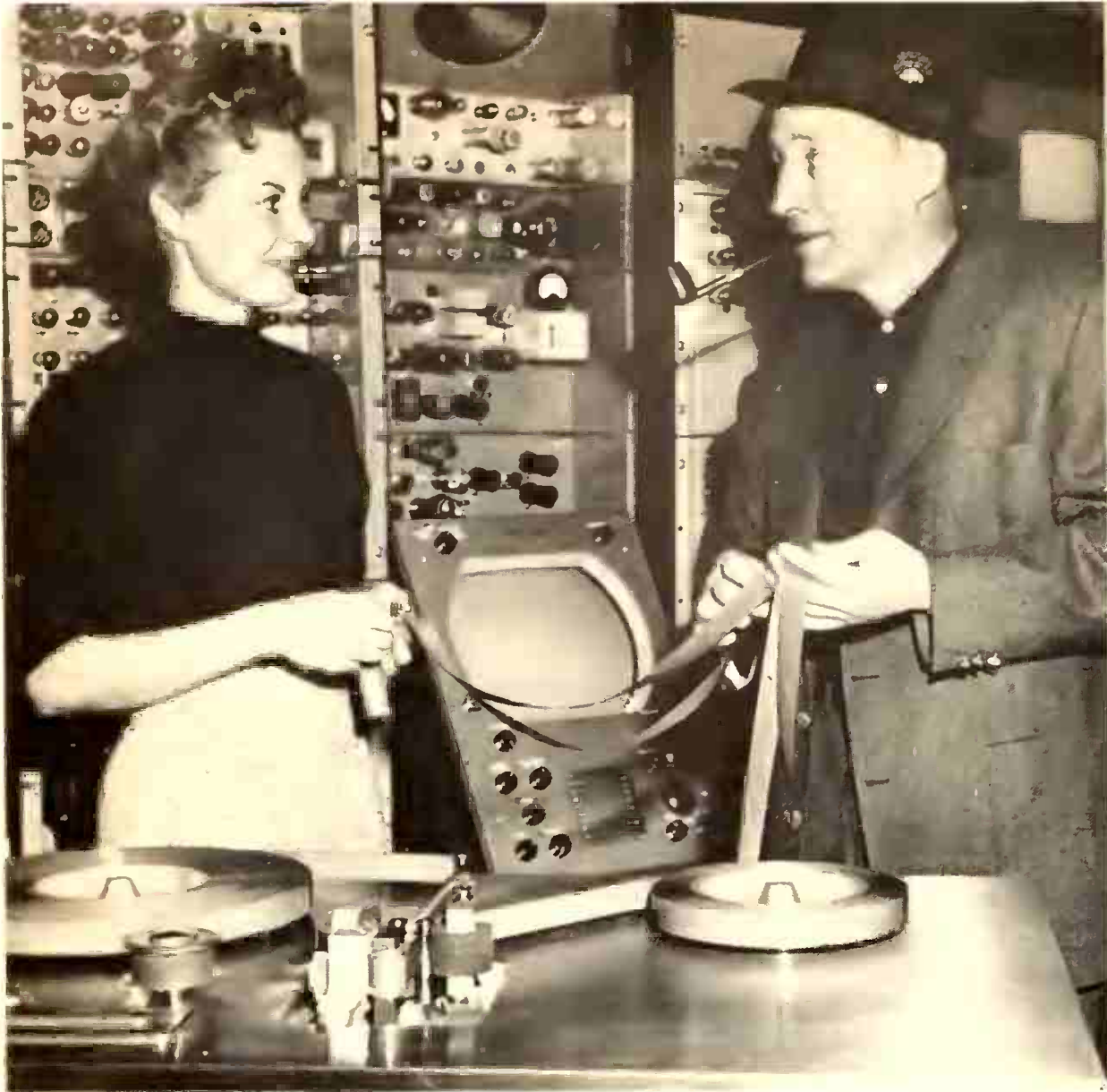
BING CROSBY: In the foreground is video tape recorder developed by Bing Crosby Enterprises, Inc. Crosby and employee handle plastic tape, now one inch wide
