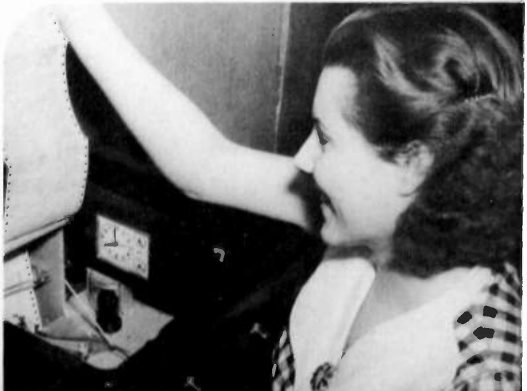
At home, your receiver picks up the signal from the air, just as your radio does, but instead of making a sound through a loudspeaker, a small stylus with a needle point "records" the tones on another strip of paper, making the loud tones blacker than the soft ones. Thus, line by line your news from the air is printed before your eyes, and removed from the machine as shown by receptionist Ruth Leffler.
