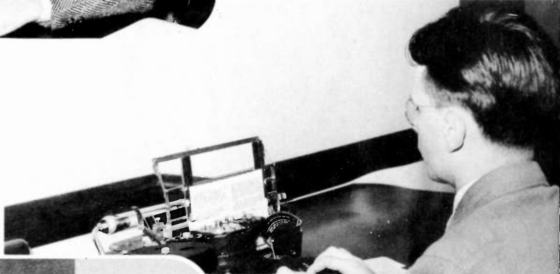
O. A. Sardi, Chief Engineer, inserts the copy into the facsimile transmitter. The black scanning head, in front of the strip of copy, converts any printed, sketched or photographic material into electrical tone signals like the impulse you receive on your radio broadcasts. The scanner, a photocell, moves from left to right across the paper. Variations of reflected light effect the volume of the signal as it goes into the air, just as you hear loud and soft tones from a voice.
