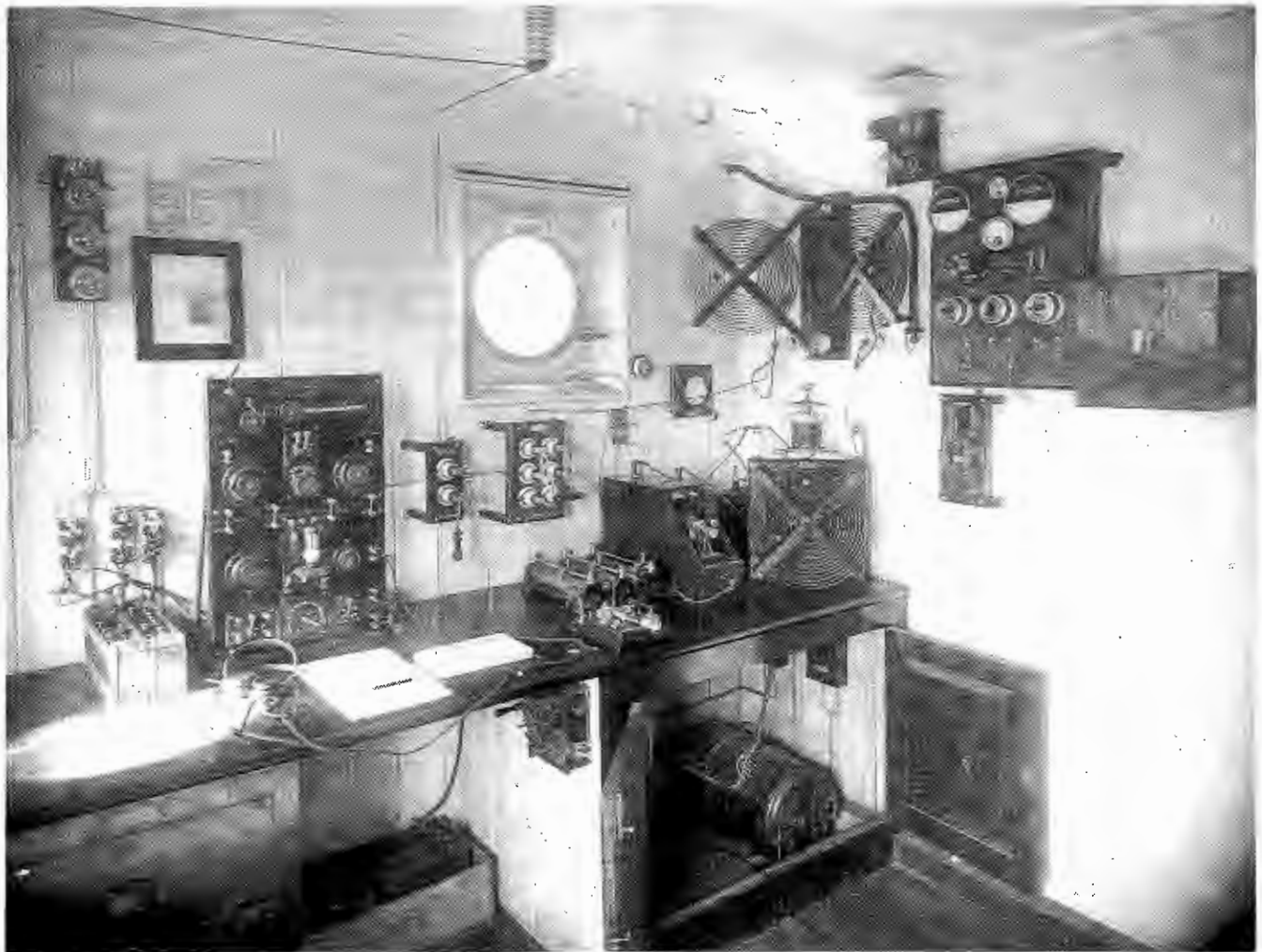
Before about 1920, 'wireless' tended to mean telegraphy ('Morse'), mainly for shipping. Here is the radio cabin of 's.s. Burwah', fitted with an AWA 500-watt quenched spark transmitter and panel receiver.
