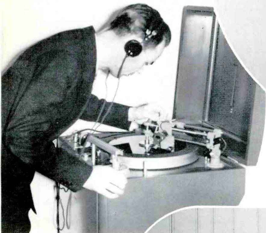
Left—Ralph Cannon is constantly alert to every advancement in radio technique. Here, he adjusts KFDA's new instantaneous recorder to "cut" a program and preserve it for future reference.
