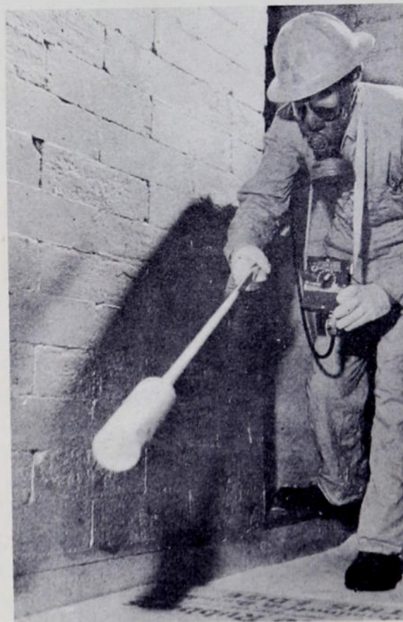
(Above) An advance monitor entering an area of high radioactive contamination. (The average individual would not require such elaborate protective devices.)
