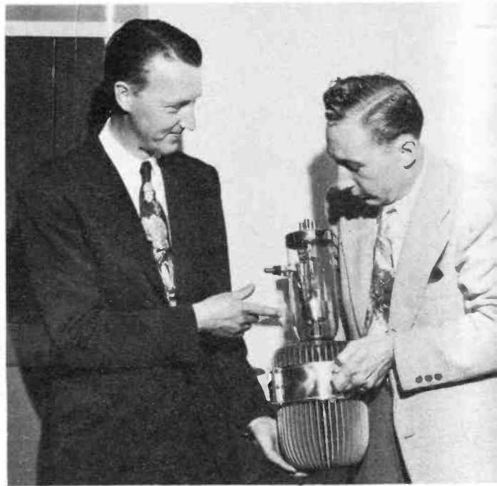
One of the sensitive and valuable air-cooled tubes used in KING's modern transmitter.
