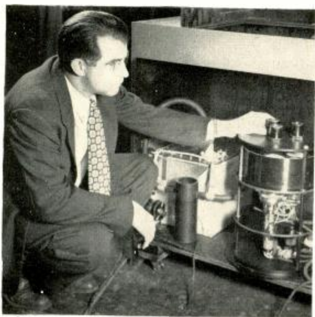
Ray D. Kell, head of television research section at the RCA laboratories, examines the Trinoscope , heart of an all-electronic color TV receiver. Those are lenses he's touching
