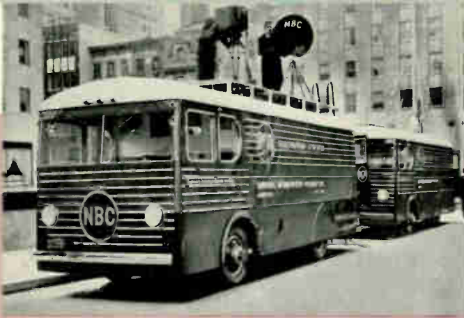
These two large motor vans house America's first mobile television station, to be used by NBC in experimental pick-ups of outdoor news events.
