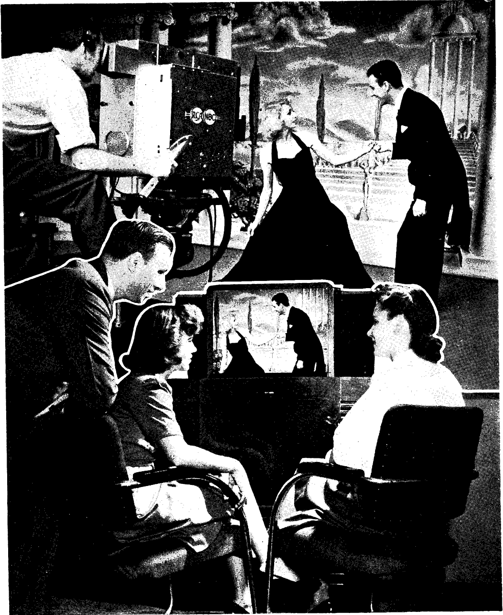
AN EXPERIMENTAL RCA ELECTRONIC TELEVISION RECEIVER WITH A SCREEN 13½ BY 18 INCHES REPRODUCES A DANCE STAGED IN THE NBC STUDIO AT RADIO CITY AND BROADCAST BY THE NBC PIONEER TELEVISION STATION WNBT, NEW YORK.
