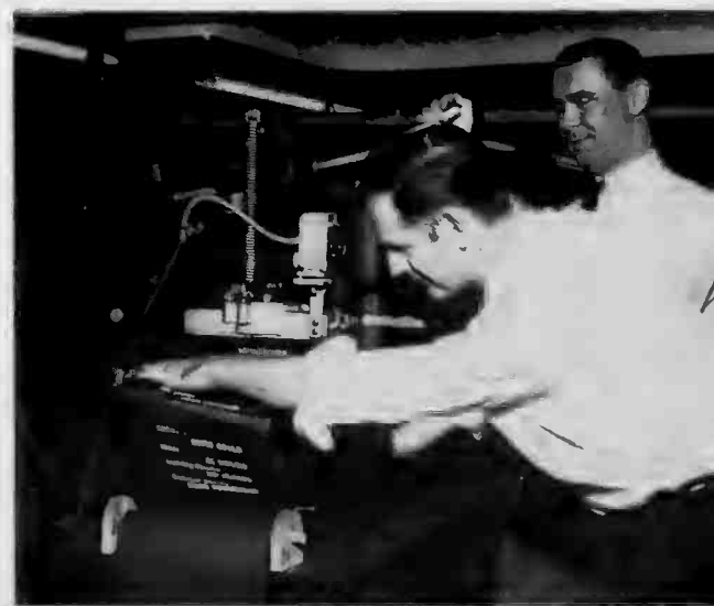
Bill Shortridge (foreground) and Dick Tibak are printing a crawl by Hot Press, white on black, to be used for a super-imposition of closing credits over a live scene.
