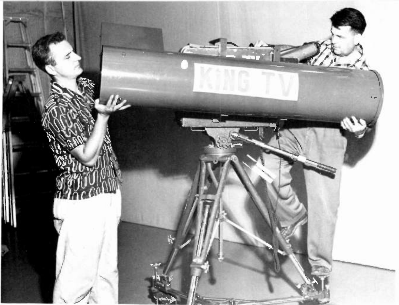
Al Smith (left) and Earl Thoms demonstrate the 40-inch telescopic lens they invented for KING-TV 's early Gold Cup race coverage. The side-mounted lens is actually an astronomical telescope using a home-ground 6-inch mirror, with smaller mirrors for coupling the image into the camera's pickup tube. Until telescopic Zoomar lenses came along, two different networks used this patented system, which grew out of Earl Thoms' long-time hobbies of lens-grinding and star-gazing.
