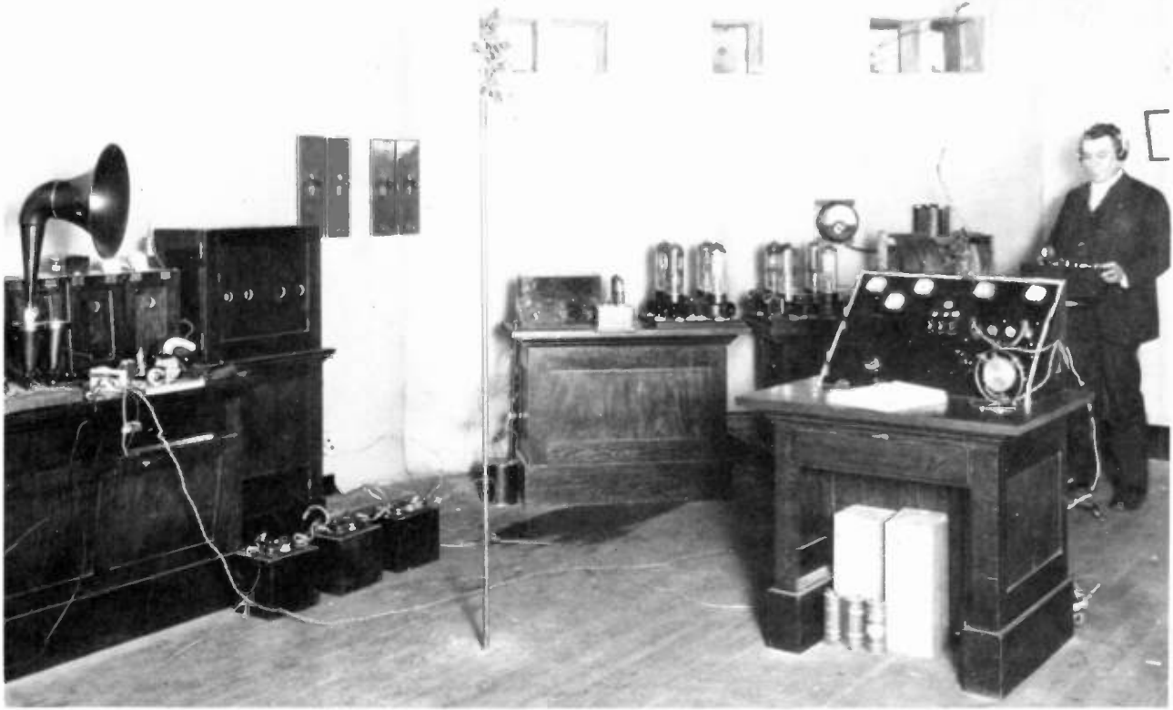
Seattle City Light Superintendent James Delmage Ross personally supervised construction of KTW for the First Presbyterian Church in 1922. This photo shows Ross (for whom Ross Dam is named) at work in the transmitter room, inside an ornamental dome high above the church roof. By this time (1925) partitions and a ceiling are in place. Earlier, the equipment was simply bolted to such beams and posts as passed through supporting the cupola.
