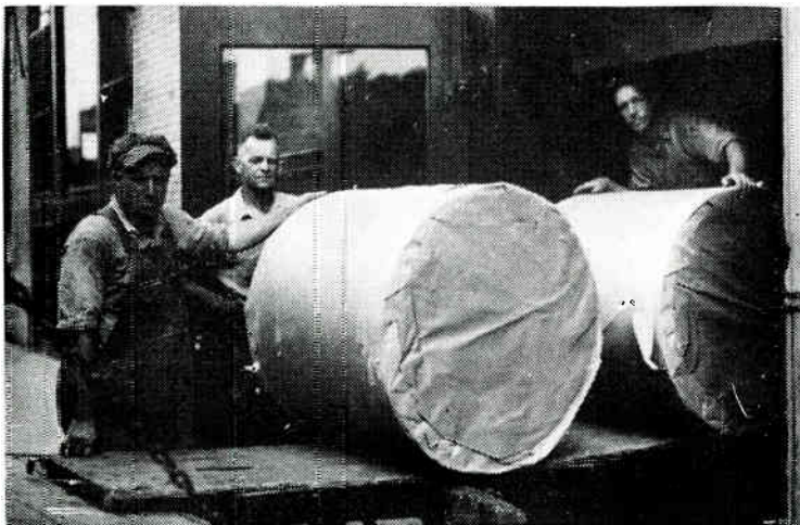
Newsprint comes to the Janesville Gazette in large rolls as shown above. These rolls weigh about 950 pounds and more than a thousand are used in a year. After the heavy brown wrapping paper has been removed from the rolls they are ready to be hoisted by an electric crane to proper position on printing press.
