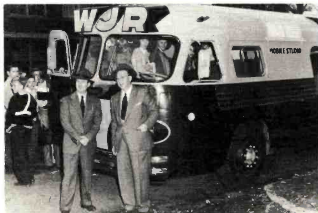
WJR's mobile unit, a self-contained radio station on wheels, travels into rural areas to originate on-the-scene broadcasts of agricultural events and local Fairs.
