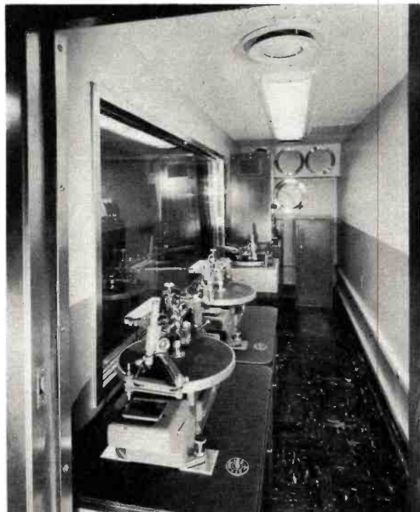
The WJR recording studio houses a battery of machines for "putting on wax" those programs slated for later broadcast.
