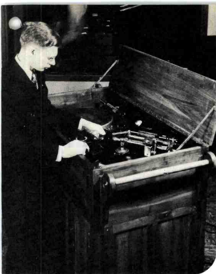
Another innovation credited to the WKBN technical staff is this compact "sound effects wagon." It is so constructed that it may be used to cut or record transcriptions; can be quickly altered to "play back" for audition purposes; can be connected to play transcriptions for broadcast, or can be used to introduce recorded sound effects during studio dramatic presentations. Its specially designed undercarriage also permits its easy transfer from one studio to another. Engineer Carl Lindberg is shown at the unusual machine.
