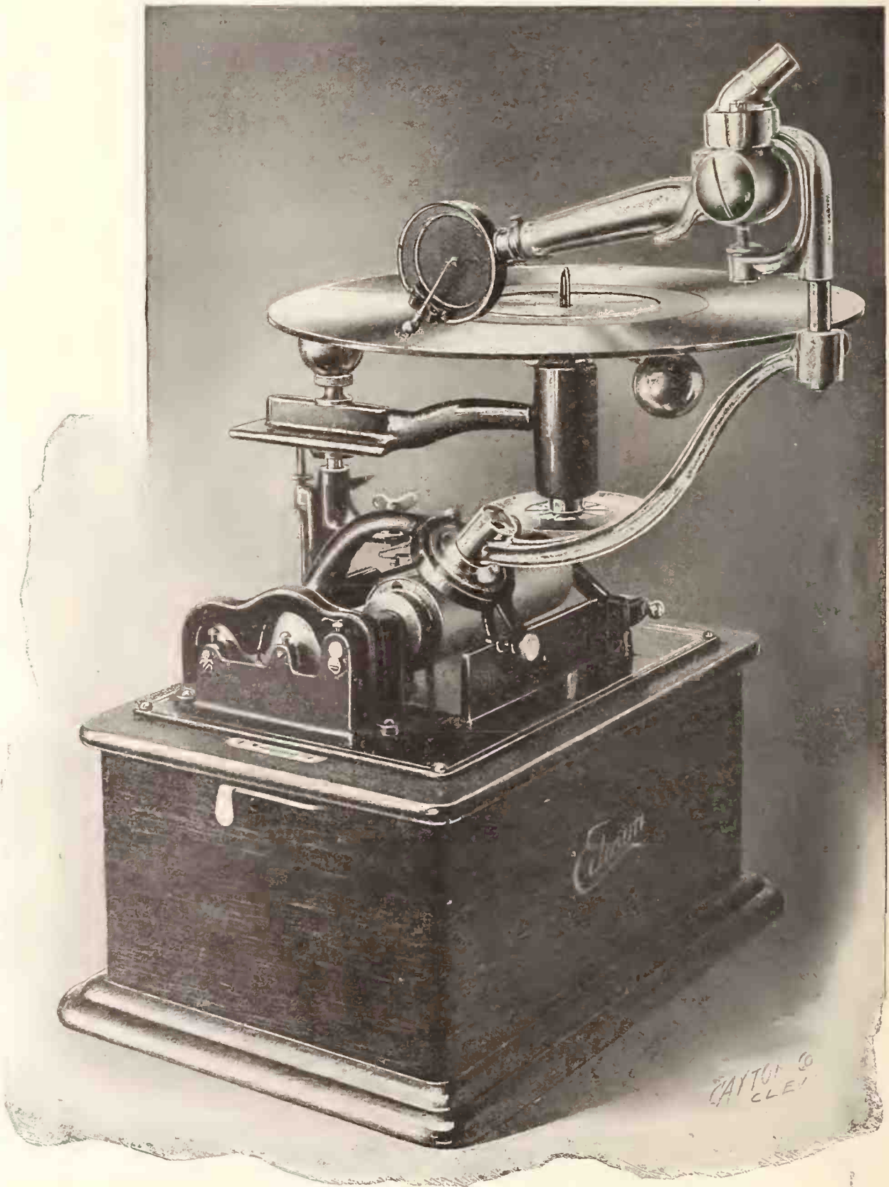
THE DEVINEAU BIOPHONE attached to a cylinder machine.
