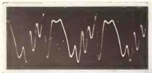
OBOE—Here we have a tone-wave which shows unmistakably a tone of very distinct individuality. The pronounced irregularities of the oboe's tone-wave are caused by the dominance of certain of its partial-tones.
