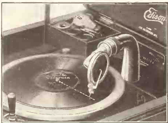
Patent Applied for Illustration shows the position for playing Victor and all other lateral cut records. Note the dotted line which shows the exact centering of the needle on the record and which prevents the reproducer from coasting when record is finished playing.
