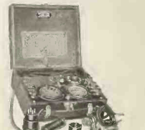
Weston 528 Set Tester ture, a small, triple-range portable AC instrument, known as the Weston model 528.
