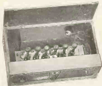
Open View—Note ready accessibility of tubes, power supply, etc.
