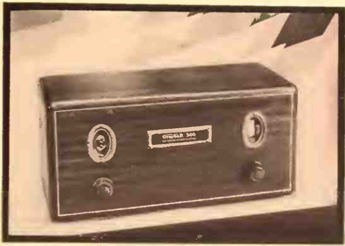
GRAYBAR 300—Single control, six-tube storage battery set, tuned radio frequency circuit. Mahogany finish cabinet.
