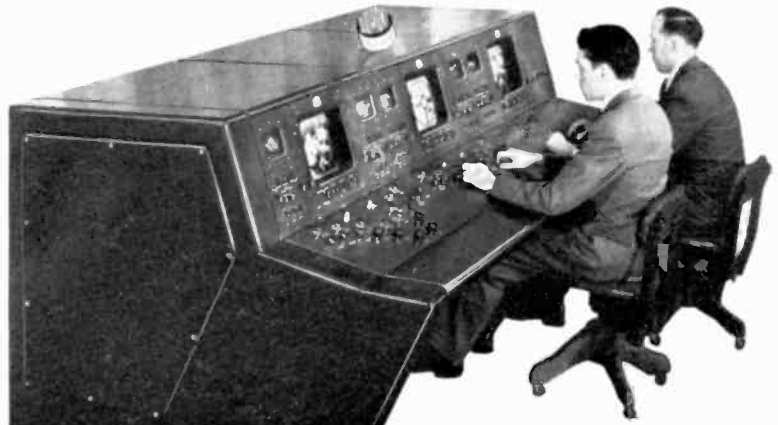
Du Mont Type TA-105-A Film Pickup Control Console. Includes saw-tooth, parabola and sine-wave shading with 5" waveform monitors for both line and frame. 12" picture monitor. Instantly accessible chassis. Integral design with the Du Mont Type TA-108-B Video Mixing Console and associated equipment which will handle four separate video or composite input channels with automatic or manual "fades" and "lap dissolves" between any video input channels.
