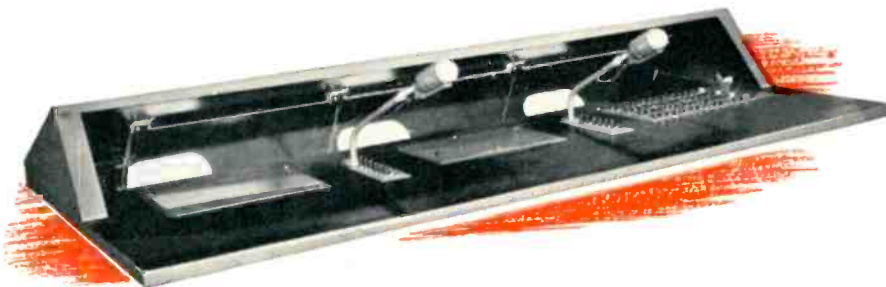
RCA Program Directors Console Type TC-5A. Television's most up-to-date directors' control. Includes large-size picture monitors for the studio outgoing line, for previewing, and for "on-the-air" monitoring. All switching under finger-tip control. Low height for full studio visibility. Recessed monitors for maximum image brightness in a fully-lighted control room.
