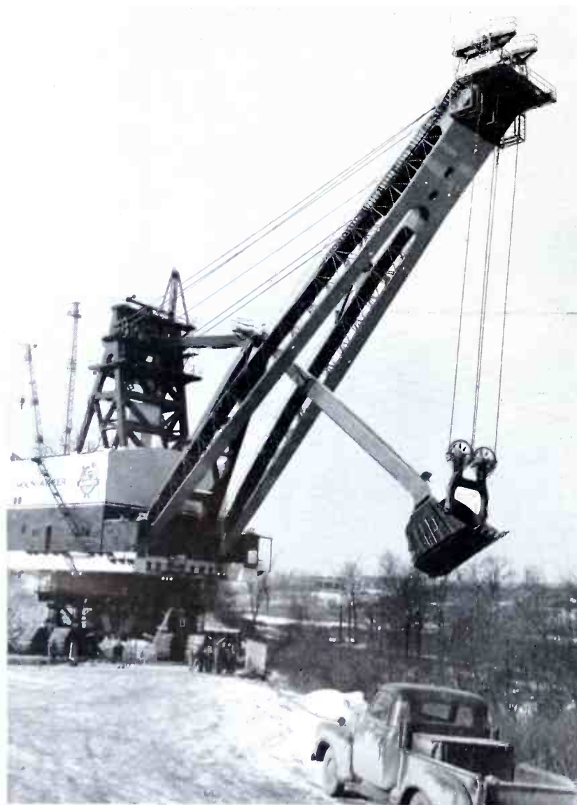
In the Wheeling area lies the nation's only natural supply of coal sufficient for power production necessary for aluminum plants in the eastern United States. Here is the world's largest strapping shovel operated by the Hanna Coal Co. New coal processes now make Ohio Valley power available at prices competitive with Hydrolic power. Projected underground mines fan out for 30 miles from the Wheeling area.
