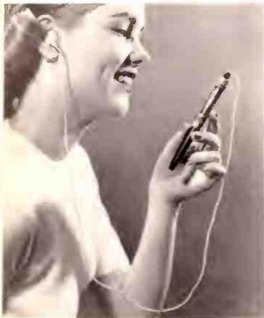
RCA has exhibited this model of a five-tube transistorized radio in a two-ounce fountain pen case that holds batteries and antenna.
