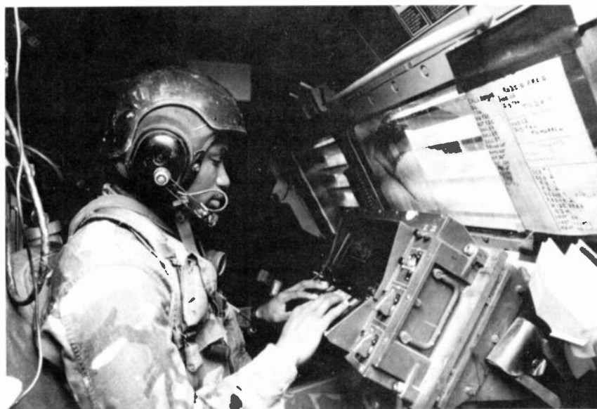
Figure 1. ( Computer: Impact—Impact on Military Affairs ) Fire control computer of the Multiple Launch Rocket System (MLRS), containing the computer that integrates the vehicle and the rocket launching operations. Courtesy of the U.S. Army, Public Information Division, Washington, D.C.
