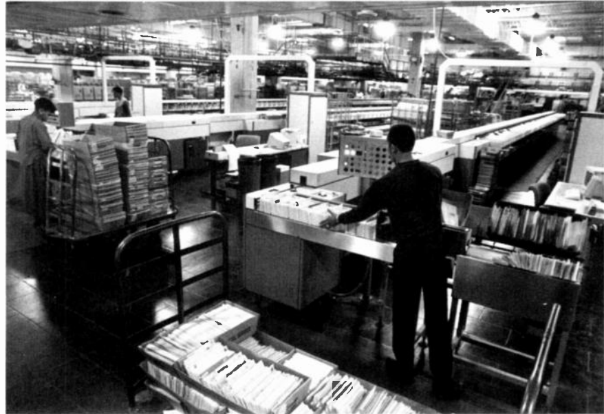
Figure 4. ( Postal Service ) A view of the general mail facility, Washington, D.C., 1986, showing two of the three optical character readers that sort thirty thousand to forty thousand letters per hour. Courtesy of the United States Postal Service.
