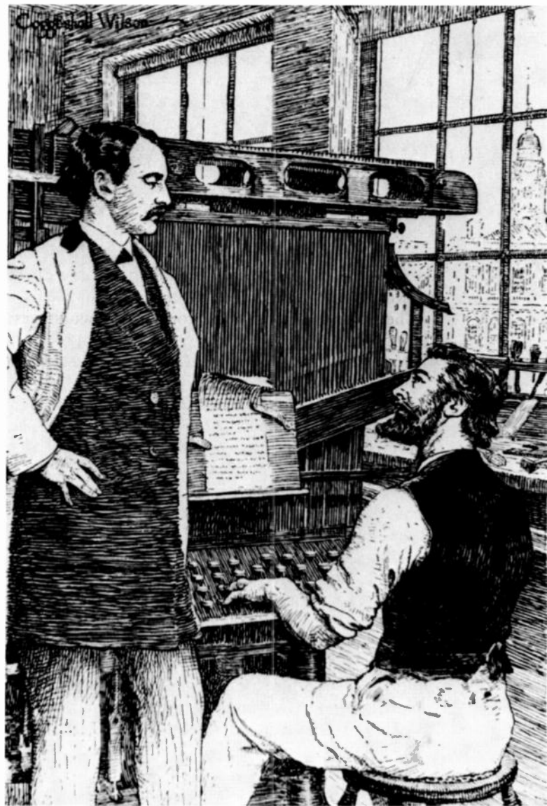
Figure 1. ( Mergenthaler, Ottmar ) Ottmar Mergenthaler demonstrating the operation of the “blower machine”—the first commercially successful Linotype—for Whitelaw Reid, in the plant of the New York Tribune . The Bettmann Archive, Inc.
