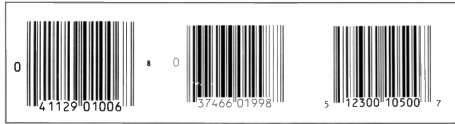
Figure 1. ( Computer: Impact—Impact on Commerce ) Examples of Universal Product Code (UPC) bar coding.
