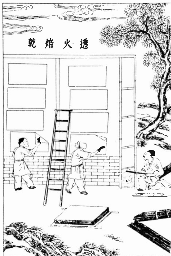
Figure 6. ( Writing Materials ) Papermaking in China. After Sung Ying Hsing. Paper sheets are dried on a wall heated by a stove (right-hand side). The Bettmann Archive, Inc.
