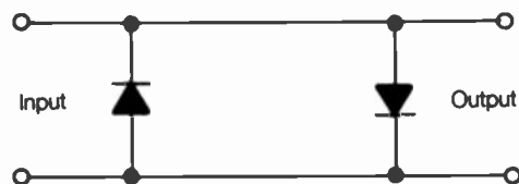
CLAMPING: Back-to-back diodes limit signal amplitude.
