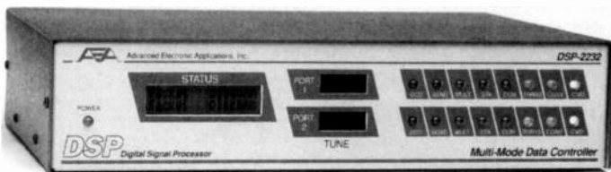
DIGITAL SIGNAL PROCESSING: A DSP multimode data controller. It interfaces the radio with a computer for digital communications. Advanced Electronic Applications, Inc.
