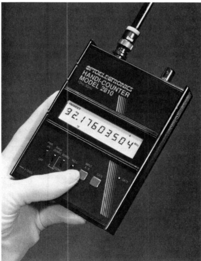
FREQUENCY COUNTER: A handheld frequency counter allows maximum versatility in the ham lab and around the station. OPTOELECTRONICS, INC. MODEL 2810
