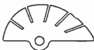
Fig. 3. End moving vane of a ganged capacitor cut into segments for capacitance matching.
