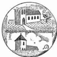
Fig. 41. Example of the effect of incorrect framing on a received television picture.
