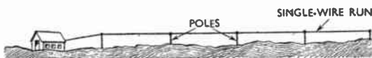
Fig. 24. Essential feature of the Beverage aerial is its great length in proportion to its height. It is commonly run on short poles in the manner of a telegraph line.
