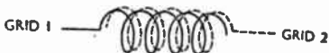
Fig. 9. Formation of the co-planar grids of the Wunderlich valve; for clarity one grid is represented in this diagram by a broken line.
