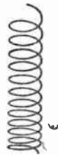
Fig. 12. The control grid of a variable-mu valve is a helix, the pitch of which changes along its length.
