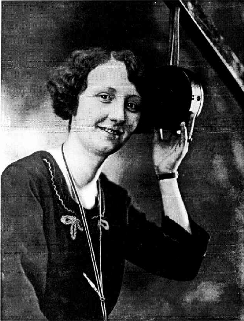
The glow-discharge microphone that was used in the broadcast of a human heartbeat.
