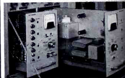
WITH . . . equipment accessibility through three drawers, three roll-out trays, two swing-open doors, one swing up panel and six main doors.
