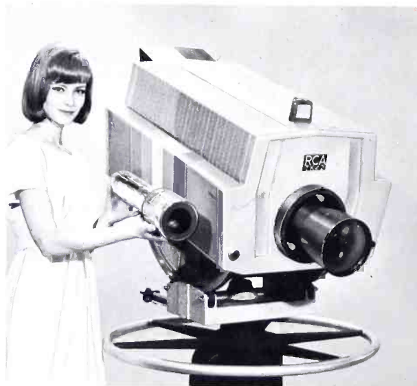
This is the 4-1/2 inch image orthicon tube used in the luminance channel to sharpen the picture.
