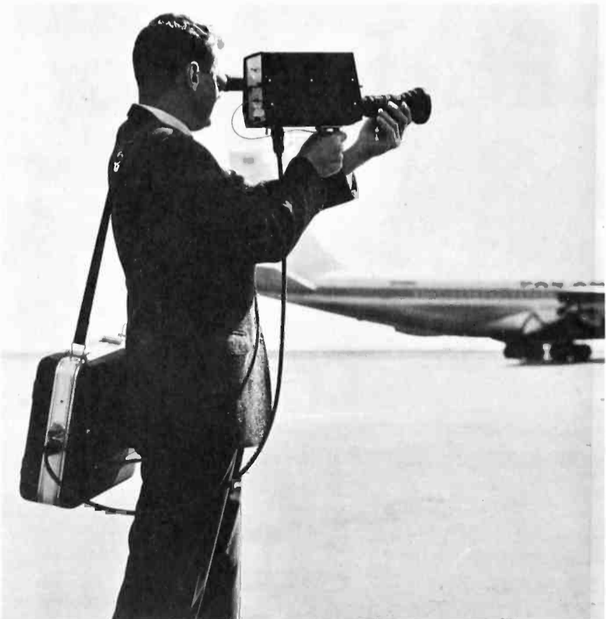
Introduced at the NAB convention in Chicago, last month, Westel's "go anywhere" camera is the world's first battery powered TV tape camera. Recording unit, in briefcase, complete with batteries and magnetic tape, weighs only 23 pounds.
