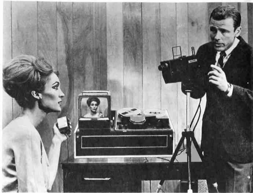
Sony home TV camera records a pretty model while her image appears on the Videorecorder screen. One inch tapes can be played back any number of times, or stored for future viewing.
