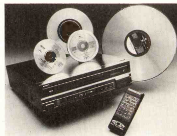
CD Video "Combi Players" have been engineered to play (foreground 1. to r.) new 5-inch gold CD Video Singles and 5-inch Compact Disc Digital Audio Discs, and (background 1. to r.) 8-inch and 12-inch LaserVision discs with either analog or digital sound.
